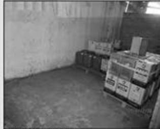
Photo of non-conformity No secondary container in chemicals warehouse.JPG
